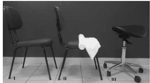
Figure 1 – The seats analyzed in the study: (I) Standard, (II) Ischial support and (III) Salli.
