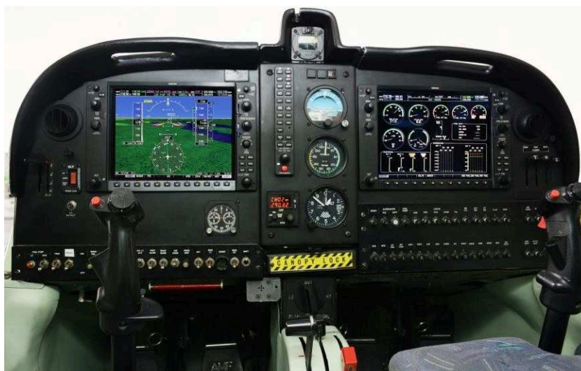
Figura 73 - Painel de instrumentos do PAC Super Mushshak ( http://kaiser-aeronaut.blogspot.com/2017/09/super-mushshak-nifty-trainer-comes-of.html ).
