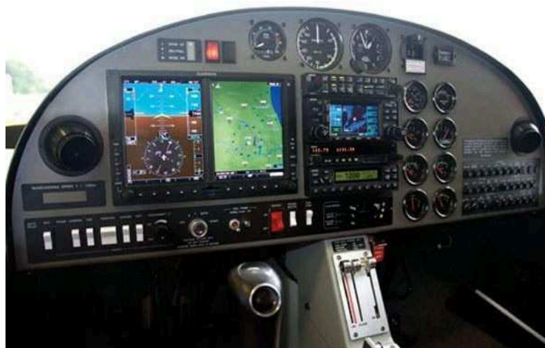
Figura 51 - Painel de instrumentos equipado com a suíte Garmin G500 ( https://www.airforce-technology.com/projects/diamond-da20-c1-utility-and-trainer-aircraft/attachment/diamond-da20-c1-utility-and-trainer-aircraft3/ ).
