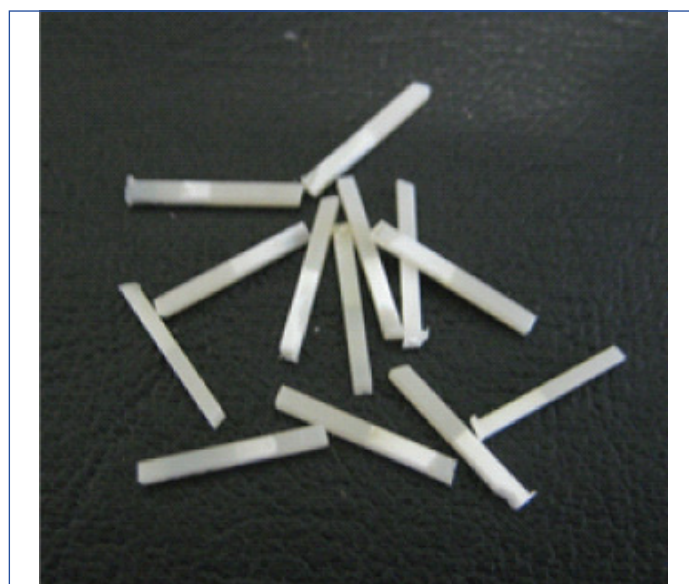
[Table/Fig-2]: The sticks used in the study that have 10 mm in length; 5 mm in dentin and 5 mm in composite resin.
