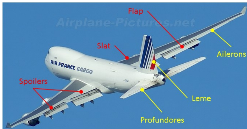
Figura 3 – Air France Cargo Boeing 747-400F – Controles de voo
